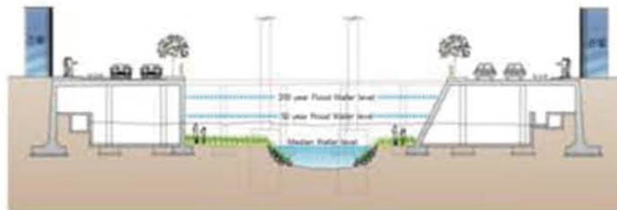
<Figure 10> Cross-section view of Cheonggyecheon and estimated flood elevation
